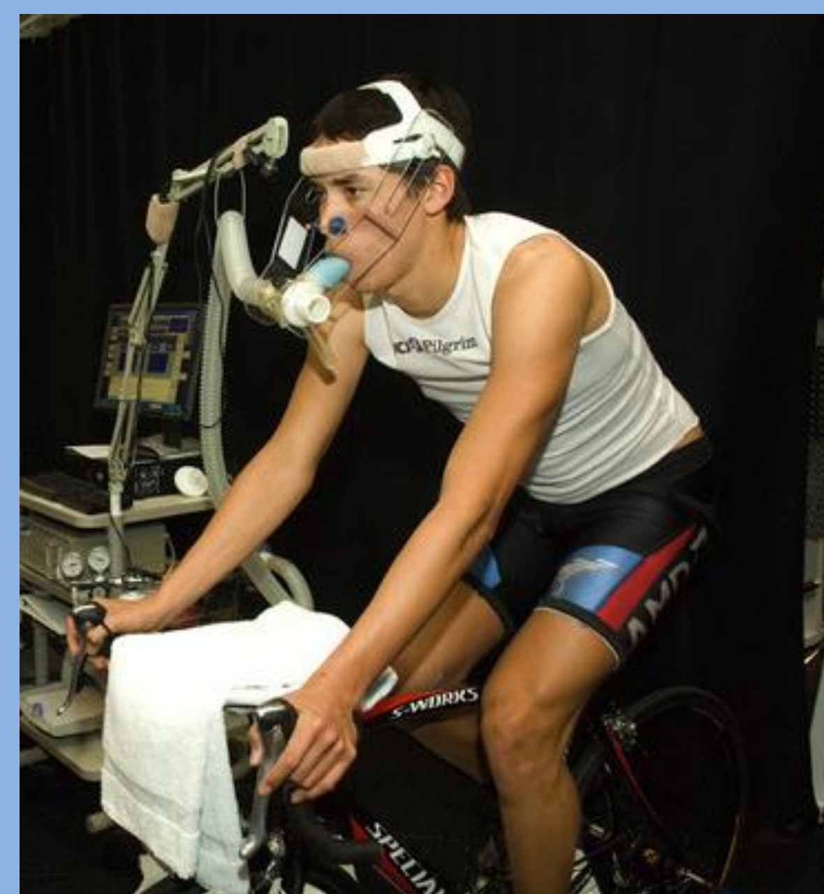
Figure 1- This system is used to collect ventilatory data to examine physiological determinants of fatigue to compare with lactate data.
