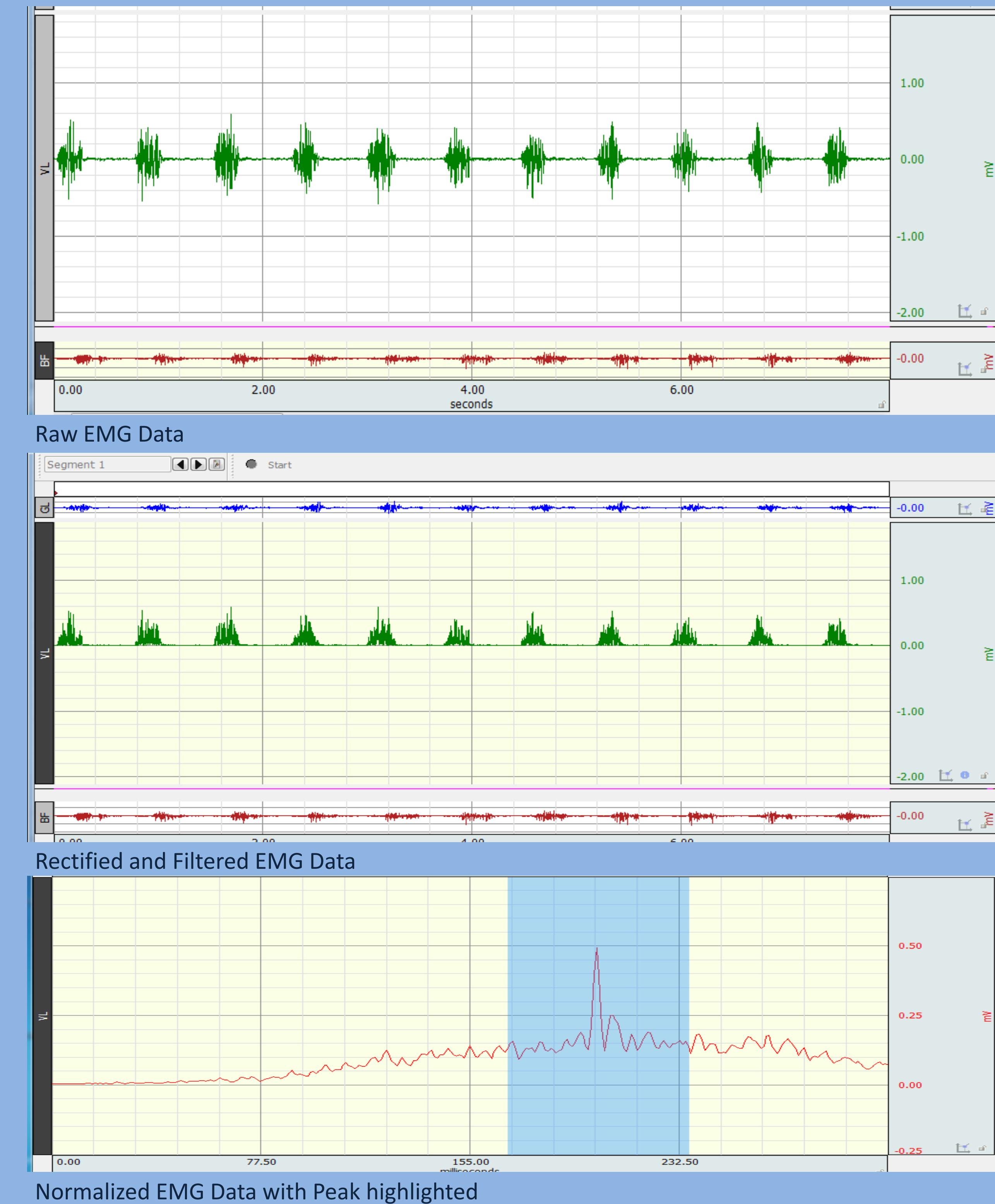
Figure 4- Raw data from the vastus lateralis is collected. It is then rectified to include all muscle activity as positive in the rest of our processing. Event markers are placed at the peaks of each pulse to identify a consistent place to measure from for normalization procedures. The data is then normalized into a graph that represents the average of the pulses, and the peak value is used for comparison between stages.
