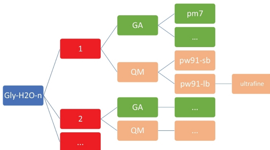
Figure 2: Representative directory structure for each cluster. The in-house scripts included in this protocol require the directory structure shown above, where n is the number of water molecules. For each n in gly-h2o-n , there are the following subdirectories: GA for genetic algorithm with a GA/pm7 directory, QM for quantum mechanics with QM/pw91-sb for PW91/6-31+G*, QM/pw91-lb for PW91/6-311++G**, and QM/pw91-lb/ultrafine for optimizations and final vibrational calculations on ultrafine integration grids. Please click here to view a larger version of this figure.
