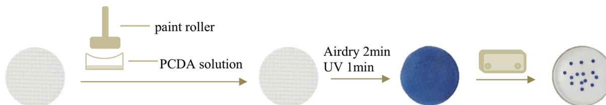
Fig. 1. Scheme of coating PCDA on filters and small discs cut from larger filter.
