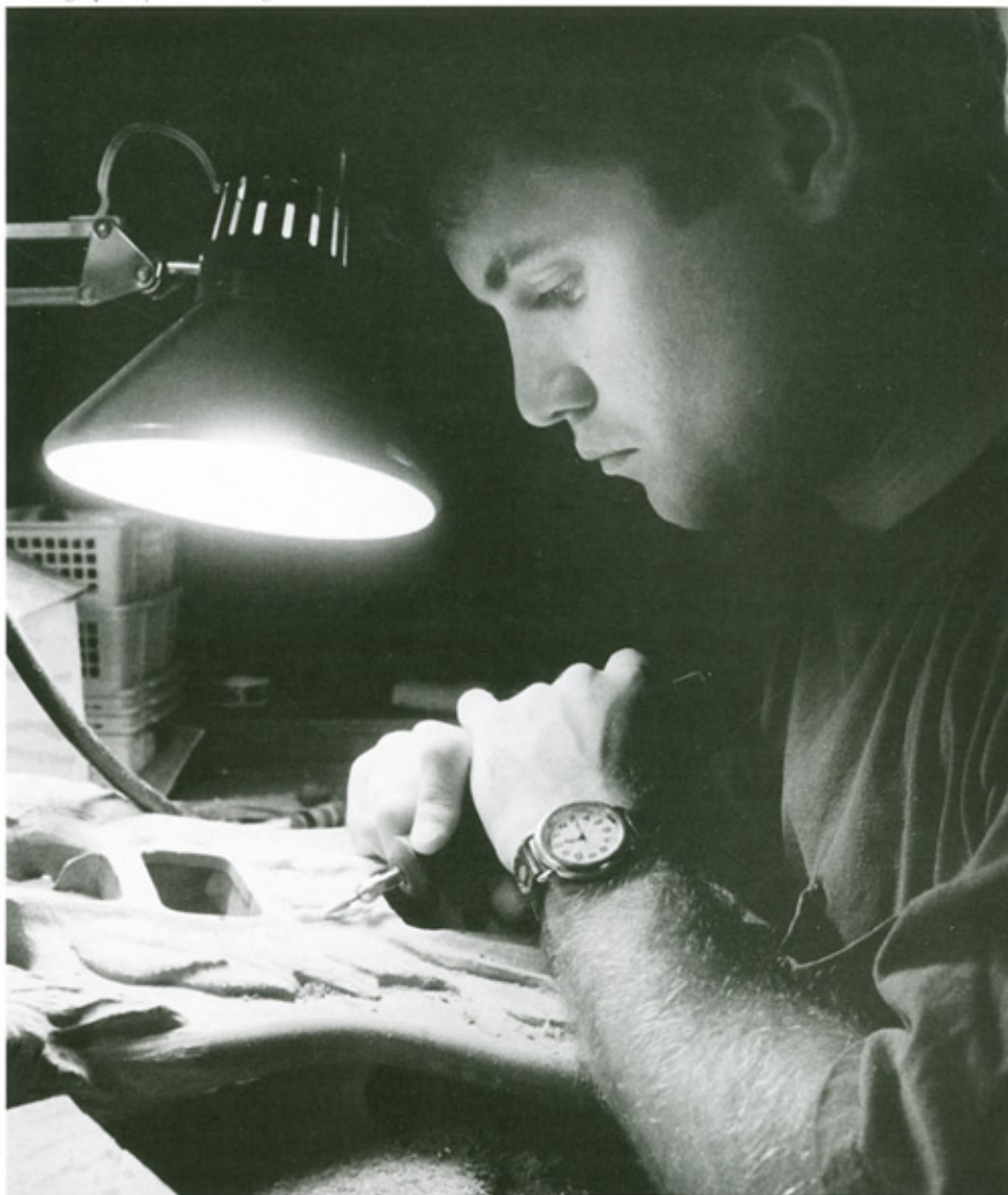
McSwain begins each project with a simple plank of wood, then spends about 10 hours contouring it into the shape of a guitar body. Carving the details takes him anywhere from 25 to 100 hours.
